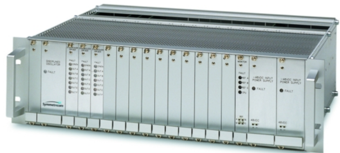
56000 Data Rate Generation and Distribution System
